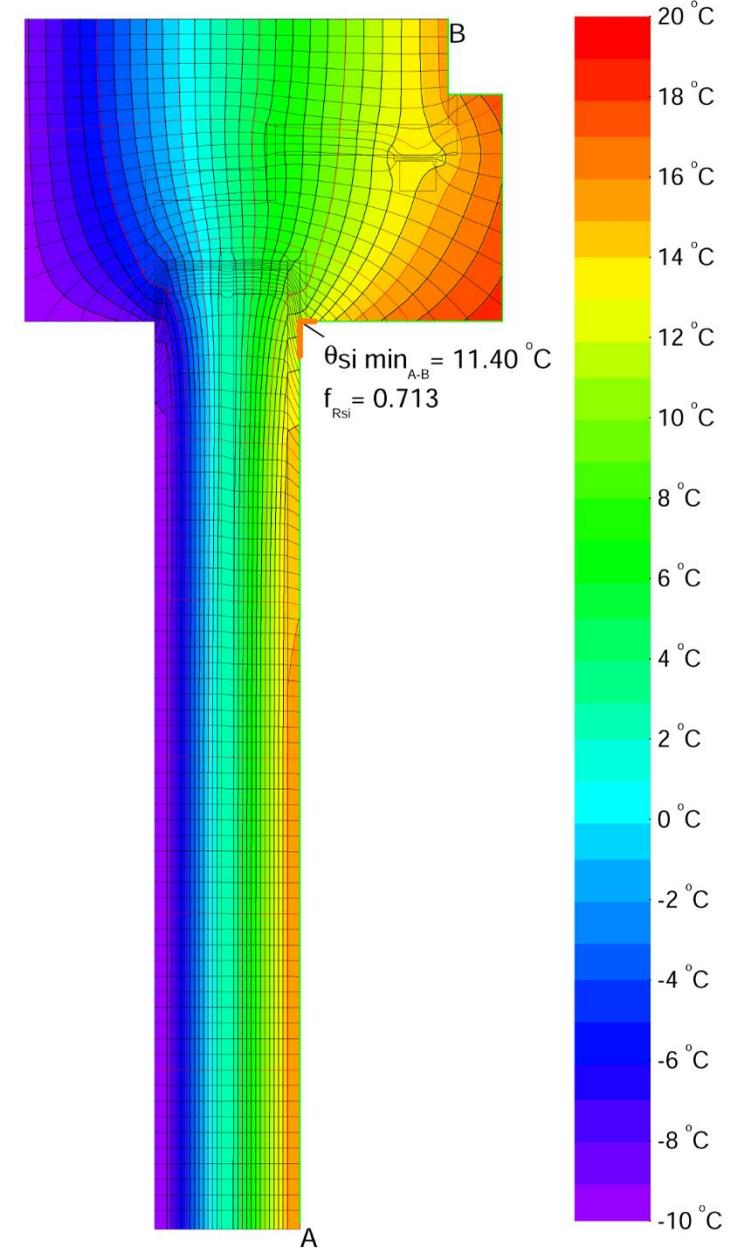
$$U_{fAB} = \frac{\frac{\Phi}{\Delta T} - U_p \cdot b_p}{b_i} = \frac{\frac{8.106}{30.000} - 0.649 \cdot 0.300}{0.100} = 0.756 \text{ W/(m}^2 \cdot \text{K)}$$
